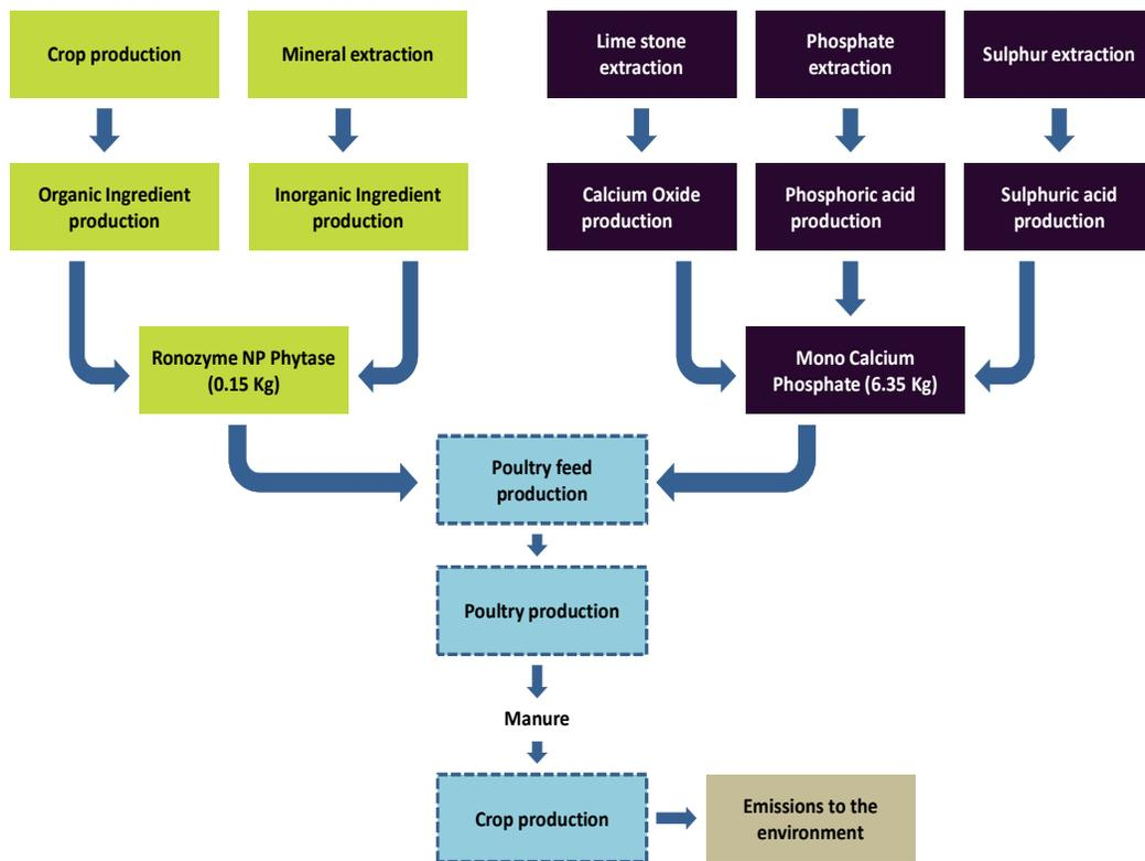
Figure 1: Main system boundaries of the study. Process indicated to the left (green) are induced process and process to the right (purple) are displaced when RONOZYME NP phytase displaces inorganic phosphorous supplementation in poultry feed. Poultry feed production; poultry production and crop production (marked with dotted boxes) are not changed when phytase displaces MCP
